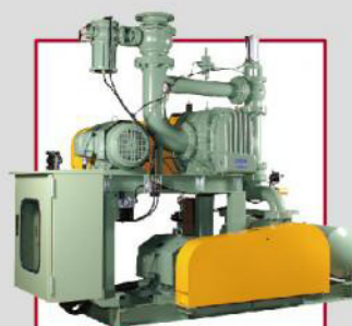
機械助力真空泵 Mechanical Booster Vacuum Pump
